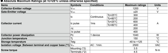
Note \*1: All terminals should be connected together when isolation test will be done.
